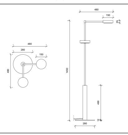
MATERIAL: Electroplated Iron/hand brushed finish LIGHT SOURCE: Integrated LED module FINISH: WATTAGE:  $2 \times 7W$ Dark brushed grey metal/brushed brass/opal white diffuser **VOLTAGE:** 230V (Other finishes available) COLOUR: 3000K **DIMENSION:** 1450mm Height 57" 17lb **NET WEIGHT:** 7.8kg Width 480mm 19" Shade dia 150mm 5.9" Base dia 280mm 11 "
