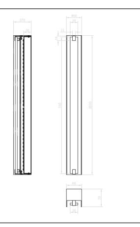
MATERIAL: LIGHT SOURCE: Integrated LED module Electroplated brass/ hand brushed finish WATTAGE: 10W FINISH: Medium bronze/ Alabaster marble **VOLTAGE:** 230V (Other finishes available) COLOUR: 3000K **DIMENSION: NET WEIGHT:** 3kg Width **IP44 RATED** 60mm 2.35" 550mm Height 21.6" Projection
